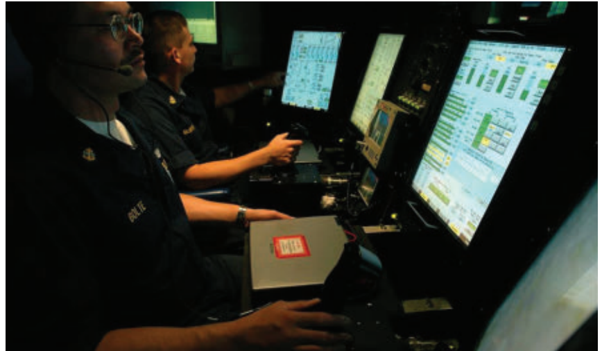
The AN/BLQ-10 provides automatic detection, classification, localization, and identification of potentially hostile radar and communications signals at sea.
