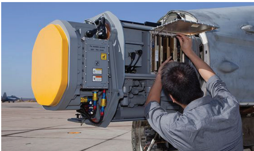
Raytheon is building six replacement AESA radar systems for Marine Corps F/A-18C/D Hornet carrier-based jet fighter-bombers.
