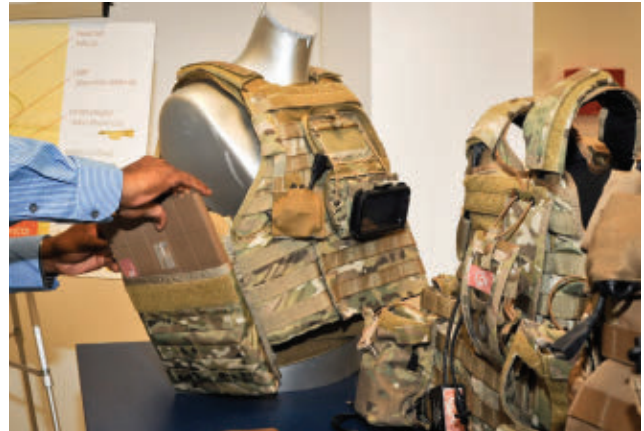
The Conformal Wearable Battery (CWB) will fit beside an infantryman's body armor, and will be able to power and recharge several different electronic devices.
